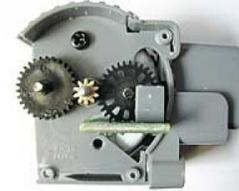
Fig. 3. Encoder Servomotor NXT (Hurbain, 2006)
