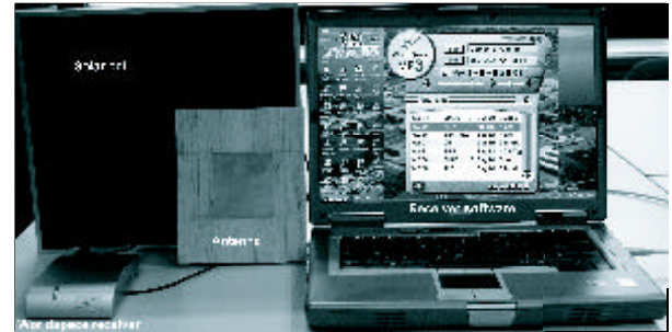
Figure 11. Worldspace signals' receiver system
