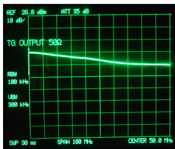
Fig. 1 The frequency response characteristic of the two-wavelength white LED.
