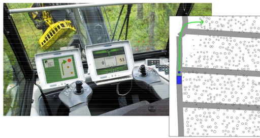
Fig. 10: “Harvester navigation to the next tree”: Is this the coming generation of harvester navigation systems which directly guide the driver to the next tree to cut. Look at the left onboard display!
