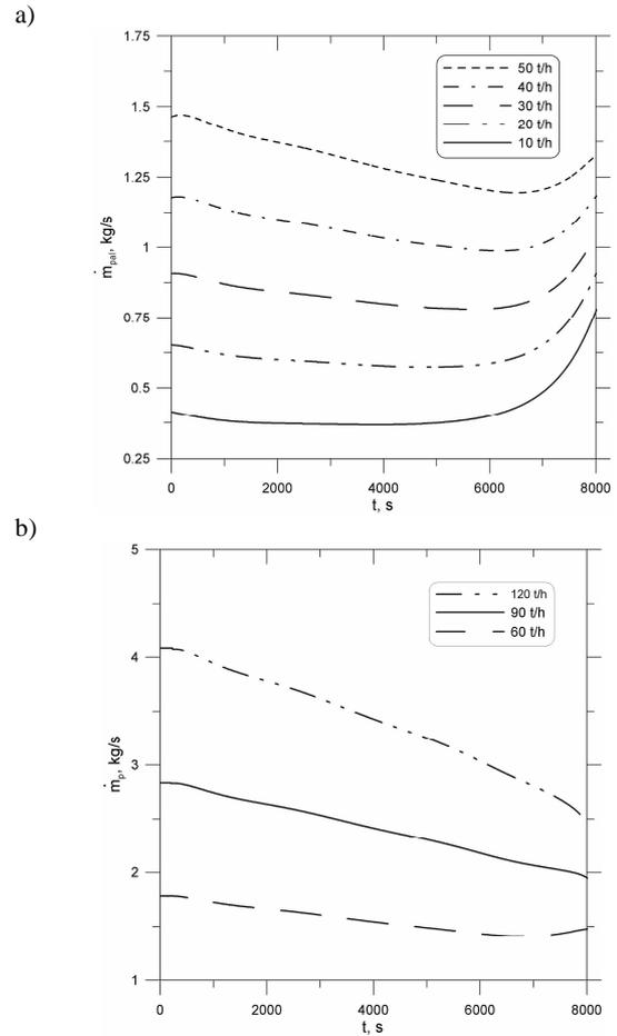
**Figure 10.** Fuel mass flow rate  $\dot{m}_{pal}$  in kg/s, during the start up of the OP-210M boiler for various mass flow rates of steam  $\dot{m}_p$  in t/h (in  $10^3$  kg/h) generated in the boiler evaporator
