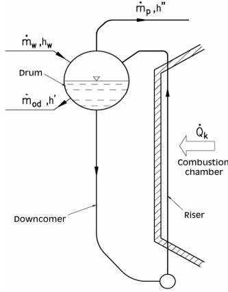
Figure 4. Diagram of the boiler evaporator
