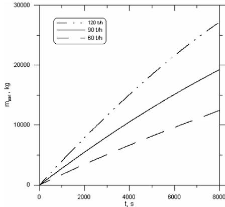
**Figure 11.** Fuel consumption  $m_{pal}$ , in kg, during the start up of the OP-210M boiler, for various steam mass flow rates  $\dot{m}_p$  in t/h (in  $10^3$  kg/h) produced in the boiler evaporator
