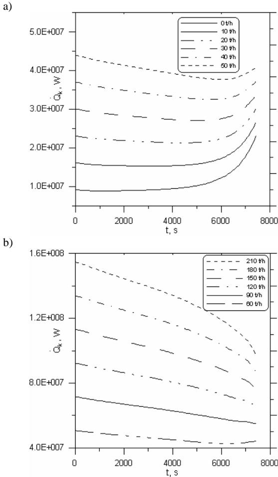
**Figure 9.** Heat flow rate  $\dot{Q}_k$  transferred to the evaporator of the boiler in the combustion chamber for various steam mass flow rates  $\dot{m}_p$  in t/h (in  $10^3$  kg/h)
