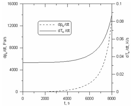
**Figure 3.** Rates of the pressure  $dp_n/dt$  and temperature  $dT_n/dt$  changes, during the evaporator heating process
