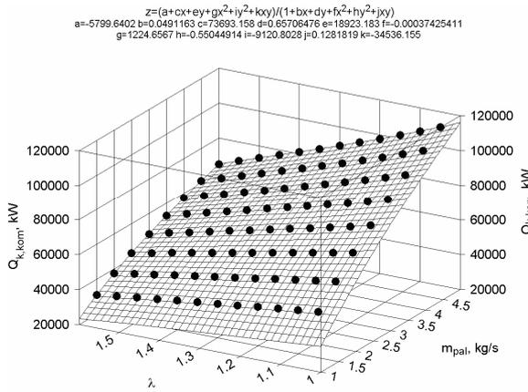
**Figure 7.** Heat flow rate  $\dot{Q}_{k,kom}$ , in kW, delivered to the evaporator of the OP-210M boiler, as a function of the fuel mass flow rate  $\dot{m}_{pal}$  in kg/s and the excess air number  $\lambda$
