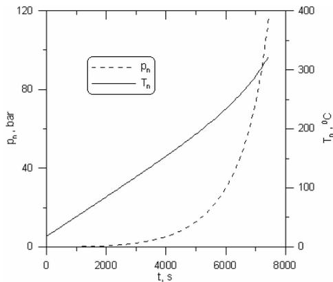
**Figure 2.** Temperature and saturation pressure changes in the boiler evaporator during the heating process
