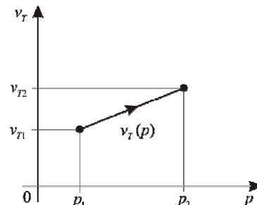
Figure 1. Heating rate of the pressure boiler element as a pressure function, determined in accordance to the TRD-301 regulations
