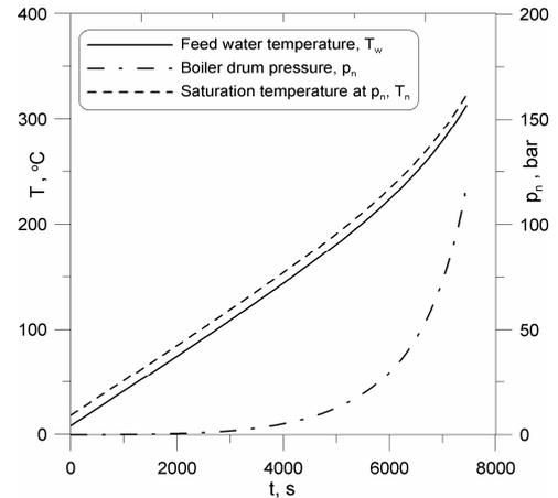
**Figure 8.** Temperature of the feed water  $T_w$ , saturation temperature  $T_n$  and pressure in the evaporator  $p_n$ , during the boiler start up
