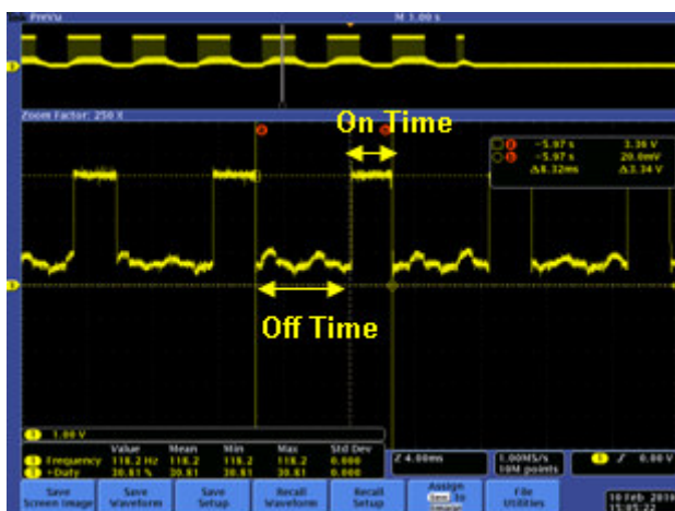
Figure 7. Oscilloscope Plot (4ms/div) Showing Voltage Applied to Disk Motors During an Individual Pulse with a 30% Duty Cycle.
