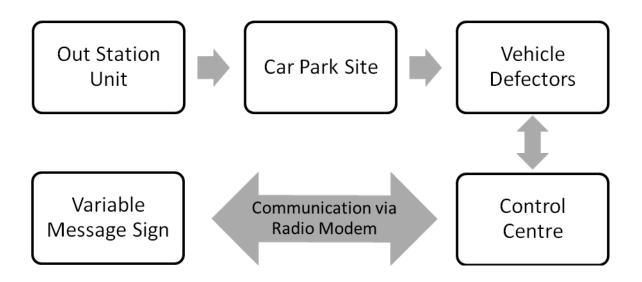
Figure 1: Conceptual Model of PGI System Operation
