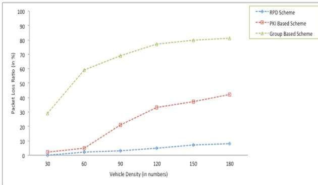
Figure 3: Message Loss Ratio vs Vehicle Density
