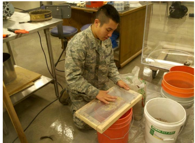
Figure 1 – Student tests a soil sieve after constructing it from wire mesh and wood
