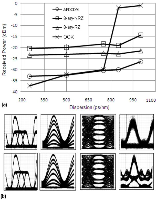
Fig.5 (a) Receiver sensitivity against system dispersion(30 Gb/s) (b) Eye diagrams at BER of  $10^{-9}$  for 30 Gb/s systems at system dispersion of 250 ps/nm (top) and 1000 ps/nm (bottom), for AP-DCDM, 8-ary NRZ and TDM (left to right)
