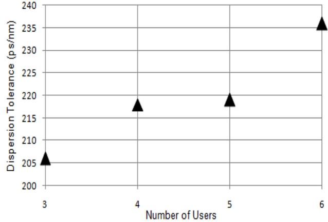
Fig. 4 Dispersion tolerance against the number of channels
