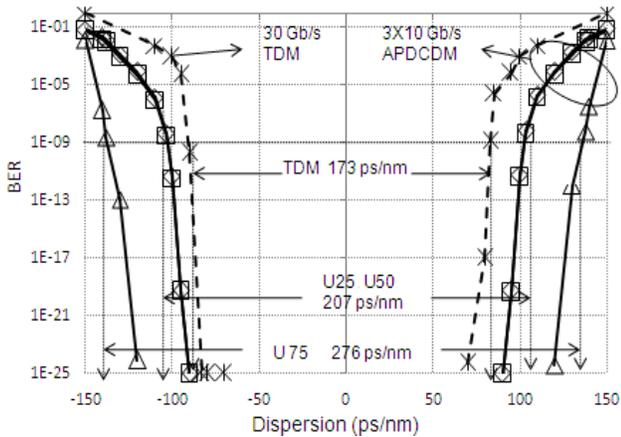
Fig. 3 Chromatic dispersion tolerance comparison between 3 x 10 Gb/s AP-DCDM and 30 Gb/s TDM at the same transmission power
