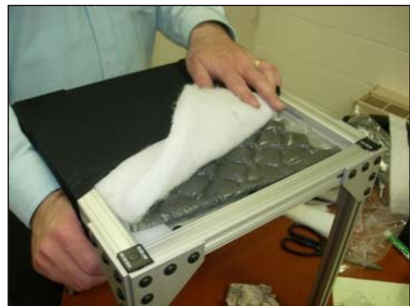
Fig. 9 Prototype with Packaged MR Fluid and Foam Layer
