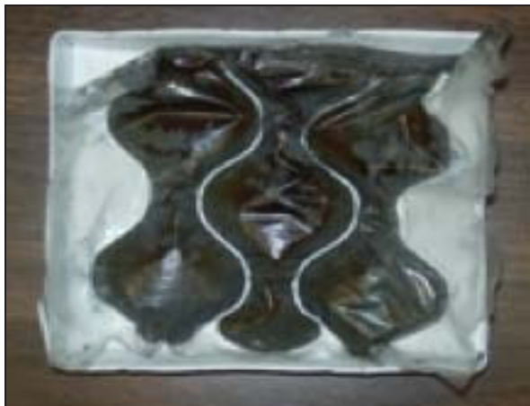
Fig. 6 Packaging Pattern for MR Fluid
