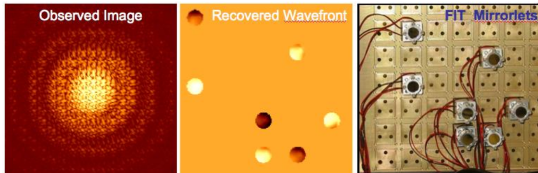
Figure 2 – Left: Observed FIT Image Center: Recovered Wavefront Right: Photo for FIT Actuated Mirrorlets
