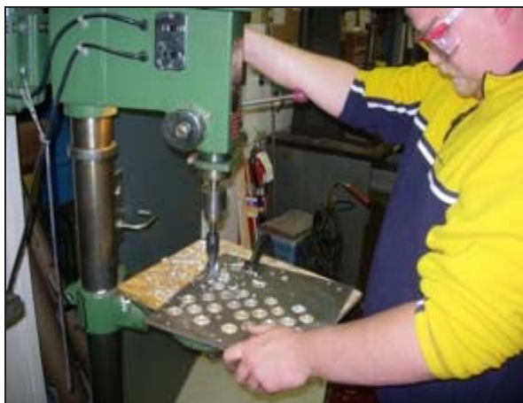
Fig. 7 Machining Magnet Placement Holes in Plate
