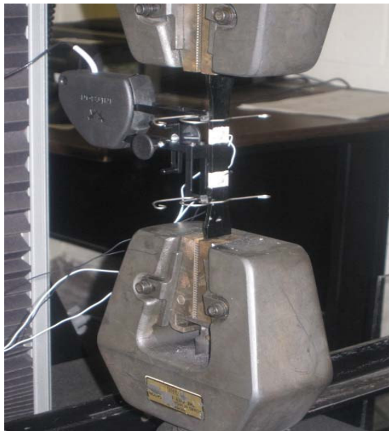
Figure 1: Specimen in the INSTRON machine with the extensometer and the electrical probes.
