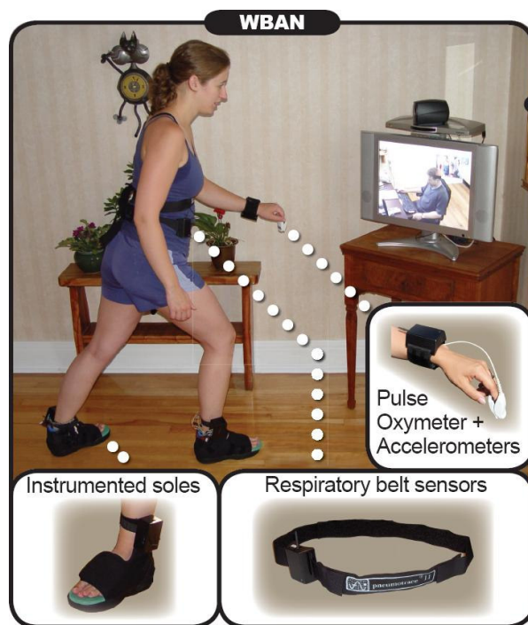
Figure 2 – Externals sensors. A computer can be included in the in-home system to accommodate several external sensors. The computer is wirelessly connected to the router and the sensor network is connected to the computer. Sensors illustrated in the picture include: inertial measurement units, respiratory belts, pulse oxymeters and instrumented soles.
