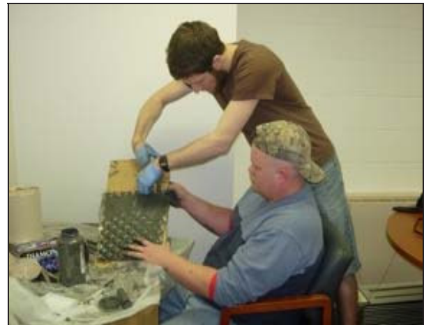
Fig. 8 Filling Packaging with MR Fluid
