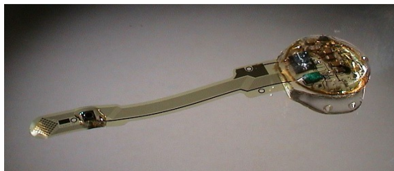
Figure 1: The retinal stimulator with its epiretinal electrode array on the left side and the encapsulated chip and energy receiving coil on the right.
