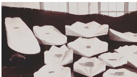
Figure 2: Principal models showing different triplets of shape, outlet location, drainage pattern, and elevation ranges.
