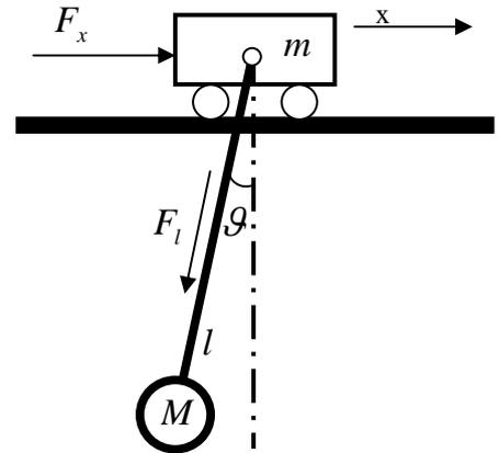
Fig.1. Schematic of the overhead crane
