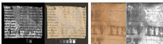
Figure 8 Image in visible light and IR - readability under a layer of paper glued to the surface of the parchment – Sg. A – 478 Figure 9 Visible light parchment vs. UV parchment (UV recording - visible patches on paper and damage to newer dates - light coloured parts)
