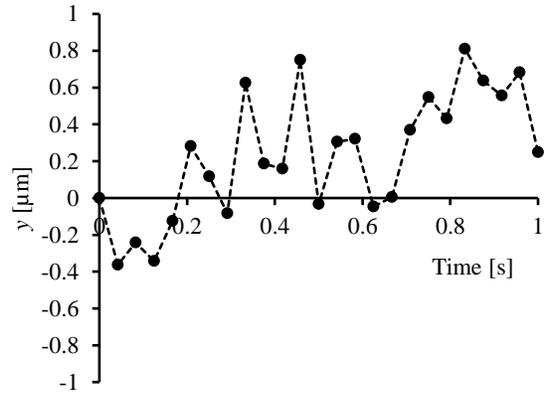
**Fig. 5:** Position tracking of micro marker (No. 1) in  $y$  direction.
