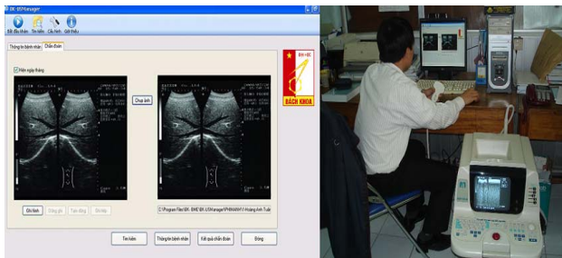
Fig.2 - Acquisition image data resulting from the software from the ultrasound machine, MEDELKOM model SLE-101M
