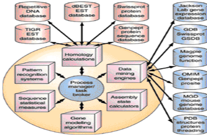
Figure 5: In the sequence analysis engine, a central task manager coordinates analysis tasks such as pattern recognition and gene modeling and also initiates sequence comparison and data mining using multiple external databases.
