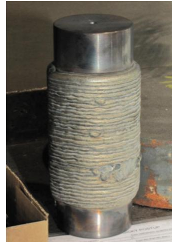
Fig. 1. Sample with welded Inconel 625
