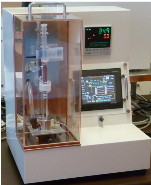
Fig. 1 Photograph of the compact-sized falling needle rheometer for measurement of fresh blood viscosity
