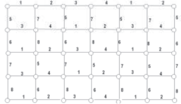
Figure 1. Optimal resource allocation for a square grid. Each of the numbers 1 to 8 represents two elements, one for each direction.
