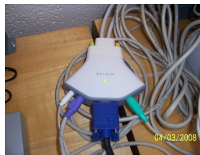
Fig. 3, KVM (keyboard, video, mouse) switch
