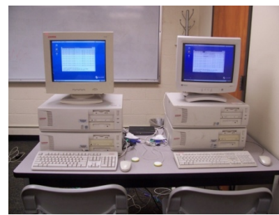
Fig. 2, Physical configuration of a 4-node cluster
