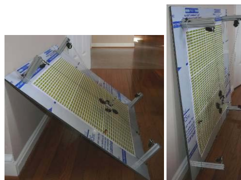
Figure 5 – Variable angles of the LOMAF showing application to sloped (left) and even vertical (right) surface access.
