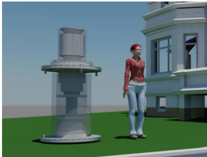
Figure 10: Idealised Flywheel Battery 20KWh Storage
